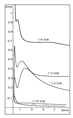
Figure 2. Chronoamperometric curves of the electropolymerization of N-phenylpyrrole (0.1 M) in acetonitrile solution containing Bu<sub>4</sub>NCF<sub>3</sub>SO<sub>3</sub> 0.1 M, on Pt electrode.
