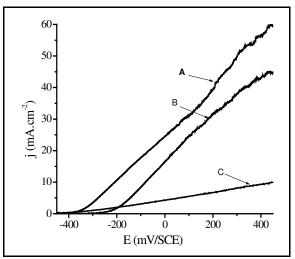
Figure 7. Polarization curves in NaCl 3% aqueous solution of naked iron substrate (A), iron substrate treated with HNO<sub>3</sub> 10 % (B) and iron substrate treated with HNO<sub>3</sub> 10 % and covered with P $\phi$ P (C) (the film was obtained by applying E = 1.2 V/SCE during 7 min).
