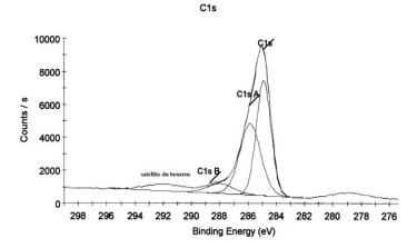
Figure 6. XPS deconvolution peaks of C1s of P $\phi$ P electrodeposited on Pt at constant potential 1.3 V/SCE (t = 5 min.).
