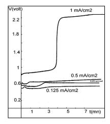
Figure 3. Chronopotentiometric curves of the electropolymerization of N-phenylpyrrole (0.1 M) in acetonitrile solution containing Bu<sub>4</sub>NCF<sub>3</sub>SO<sub>3</sub> 0.1 M on Pt electrode.
