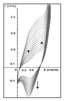
Figure 4b. Voltammograms of the growth of PφP after 5 cycles in acetonitrile solution containing 0.1 M of N-phenylpyrrole and 0.1 M of Bu<sub>4</sub>NCF<sub>3</sub>SO<sub>3</sub> on a Fe electrode. Scan rate: 100 mV/s.
