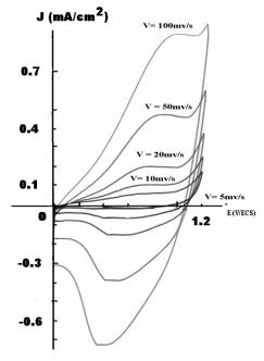
Figure 5. Electroactivity in acetonitrile solution containing Bu<sub>4</sub>NCF<sub>3</sub>SO<sub>3</sub> 0.1 M of a P $\phi$ P film obtained on Fe by the cyclic voltammetry (20 cycles).
