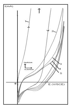
Figure 4a. Voltammograms of the growth of P $\phi$ P (1-5 cycles) in acetonitrile solution containing 0.1 M of N-phenylpyrrole and 0.1 M of Bu<sub>4</sub>NCF<sub>3</sub>SO<sub>3</sub> on a Fe electrode. Scan rate: 100 mV/s.
