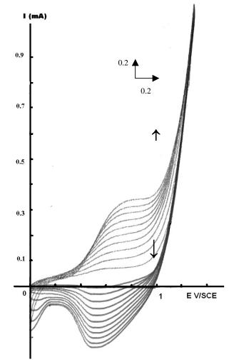
Figure 1. Voltammogramms of the electropolymerization of N-phenylpyrrole (0.1 M) in acetonitrile solution containing  $Bu_4NCF_3SO_3$  0.1 M at v = 100 mV/s on Pt electrode.
