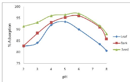
Figure 5. Effect of pH on Ni(II) removal (30 mg/L, 1.5 g leaf, 250 rpm agitation speed, 90 min. time and room temperature for leaf, at 20 mg/L, 2 g bark, 250 rpm agitation speed, 120 min. time and room temperature for bark and also at 50 mg/L, 2.5 g seed, 300 rpm agitation speed, 90 min. time and room temperature for seed adsorbent).
