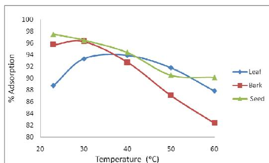
Figure 6. Effect of temperature on Ni(II) removal (30 mg/L, 1.5 g leaf, 250 rpm agitation speed, 90 min time and pH of 5 for leaf, at 20 mg/L, 2 g bark, 250 rpm agitation speed, 120 min time and pH of 6 for bark and also at 50 mg/L, 2.5 g seed, 300 rpm agitation speed, 90 min time and pH of 6 for seed).
