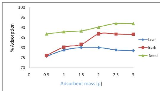
Figure 2. Effect of adsorbent dose on Ni(II) removal (room temperature, pH of 2.5, 250 rpm agitation speed and 60 min contact time for each adsorbent and also concentrations of 30, 20 and 50 mg/L for leaf, bark and seed respectively).
