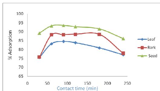
Figure 4. Effect of contact time for Ni(II) removal (30 mg/L, 1.5 g leaf, pH of 2.5, 250 rpm agitation speed and room temperature for leaf, at 20 mg/L, 2 g bark, pH of 2.5, 250 rpm agitation speed and room temperature for bark and also at 50 mg/L, 2.5 g seed, pH of 2.5, 300 rpm agitation speed and room temperature for seed).
