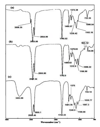
Figure 1. FTIR spectra of sunflower oil (a), epoxidized oil (b), and acetylated oil (c).
