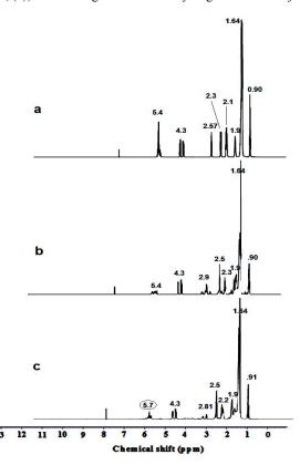
Figure 2. NMR spectra of sunflower oil (a), epoxidized oil (b), and acetylated oil (c).
