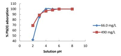
Figure 2. Effect of pH on Pb(II) adsorption onto AlSiM (m = 150 g/L; t = 60 min;  $[Pb^{2+}]$  = 66.0 mg/L, 490 mg/L; T = 298±0.5 K).
