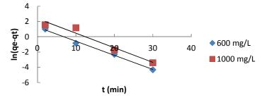
Figure 6. Lagergren's pseudo-first-order kinetics model for Pb(II) adsorption onto AlSiM (pH = 4.5; m = 150 g/L;  $[Pb^{2+}] = 600$  m/L and 1000 mg/L; T = 298 K).
