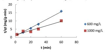
Figure 7. Lagergren's pseudo-second-order kinetics model for Pb(II) adsorption onto AlSiM (pH = 4.5; m = 150 g/L; [Pb<sup>2+</sup>] = 600 mg/L and 1000 mg/L; T = 298 K).
