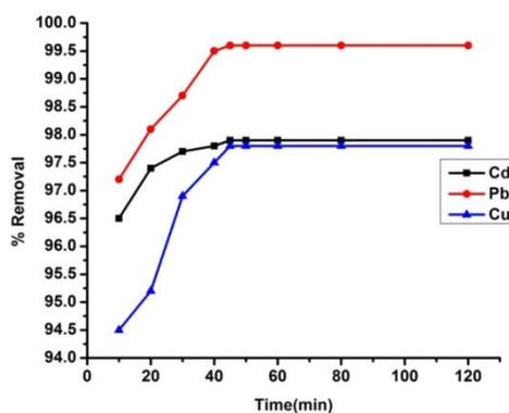
Figure 5. Effect of contact time on Cd(II), Pb(II) and Cu(II) adsorption.
