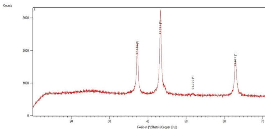
Figure 1. Powder XRD pattern of chromium doped NiO nanostructure.
