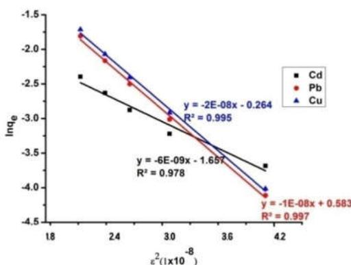
Figure 11. D-R adsorption isotherm of Pb(II), Cd(II) and Cu(II) onto Cr doped NiO nanostructure
