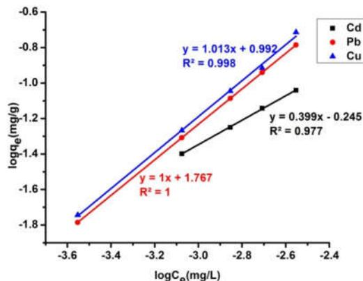
Figure 9. Freundlich adsorption isotherm of Pb(II), Cd(II) and Cu(II) onto Cr doped NiO nanostructure.
