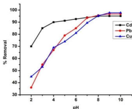
Figure 4. Effect of pH on Cd(II), Pb(II) and Cu(II) adsorption.
