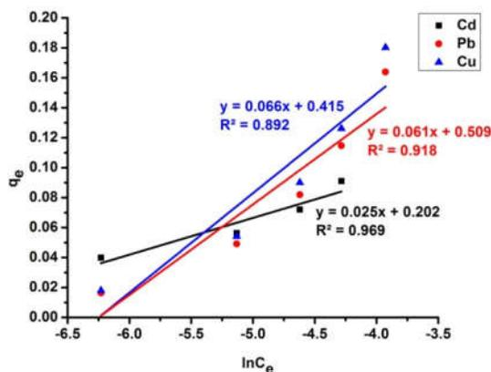
Figure 10. Temkin adsorption isotherm of Pb(II), Cd(II) and Cu(II) onto Cr doped NiO nanostructure
