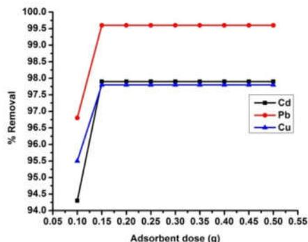
Figure 6. Effect of adsorbent dose on Cd(II), Pb(II) and Cu(II) adsorption.
