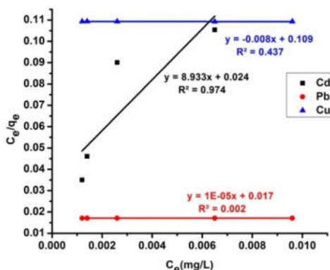
Figure 8. Langmuir adsorption isotherm of Pb(II), Cd(II) and Cu(II) onto Cr doped NiO nanostructure.
