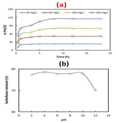
Figure 2. (a)Effect of contact time and initial concentration and (b) solution pH on the removal of carbofuran (%) onto BAS-AC at 303 K.
