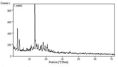
Figure 3. XRD pattern of compound 2 nanoparticles.
