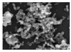
Figure 2. Field emission scanning electron microscope image of NiFe<sub>2</sub>O<sub>4</sub> nanoparticles.
