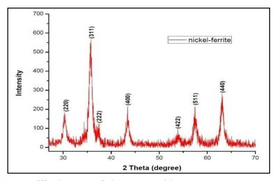
Figure 1. X-Ray diffraction pattern of NiFe<sub>2</sub>O<sub>4</sub> nanoparticles.
