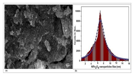
Figure 3. (a) High-resolution transmission electron microscopy image of NiFe<sub>2</sub>O<sub>4</sub> nanoparticles and (b) particle size distribution curve.
