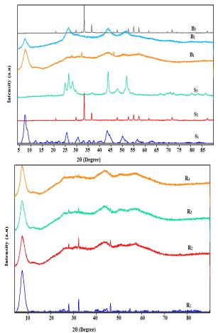
Figure 1. XRD patterns of  $S_1$ ,  $S_2$ ,  $S_3$ ,  $B_1$ ,  $B_2$ ,  $B_3$ ,  $R_1$ ,  $R_2$ ,  $R_3$  and  $R_4$  where,  $S_1 = UiO-66$ ,  $S_2 = Ag_3PO_4$ ,  $S_3 = CdS$ ,  $B_1 = Ag_3PO_4/UiO-66$ ,  $B_2 = CdS/UiO-66$  and  $B_3 = CdS/Ag_3PO_4$ ,  $R = (CdS-UiO-66-Ag_3PO_4)$ .
