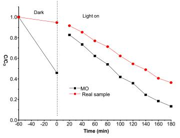
Figure 10. Photocatalytic degradation of MO and real textile wastewater using  $R_4$  (sorptiondesorption equilibrium is done for 1 h before the photocatalysis is initiated).
