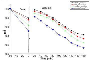
Figure 9. Degradation rate of MO as function of irradiation time in the absence and presence of scavengers (sorption-desorption equilibrium is done 1 h before the photocatalysis is initiated).
