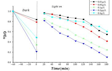
Figure 8. The effect of catalyst loading on photocatalytic activities of as synthesized nanocomposite with respect to irradiation time (sorption-desorption equilibrium isdone or 1 h before the photocatalysis is initiated).
