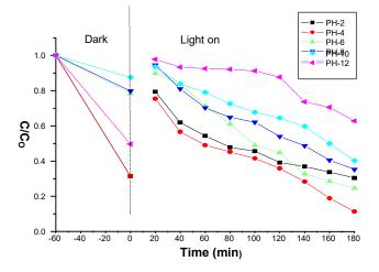
Figure 7. The effect of pH on the degradation of MO as function of irradiation time with a catalyst loading of 0.2 g/L and concentration of MO of 10 mg/L under visible-light (sorption-desorption equilibrium is done 1 h before the photocatalysis is initiated).
