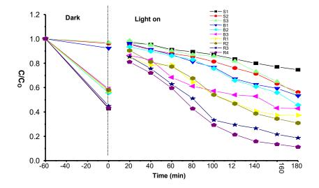
Figure 6. Comparison of photocatalytic activities of as-synthesized single, binary and ternary photocatalysts (Sorption-desorption equilibrium is done for 1 h before the photocatalysis is initiated).
