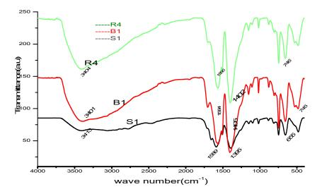
Figure 4. FTIR spectrum of synthesized nanocomposite S<sub>1</sub> (UiO-66), B<sub>1</sub> (Ag3PO4/UiO-66) and R<sub>4</sub> (CdS/Ag<sub>3</sub>PO<sub>4</sub>/UiO-66).
