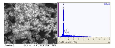
Figure 3. SEM-EDX images of the selected ternary composites R<sub>4</sub>.
