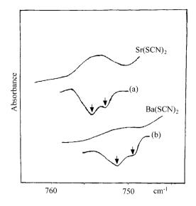
Figure 1. The second derivative of the v(CS) region of the Raman spectra of strontium thiocyanate at R = 45 and (b) barium thiocyanate at R = 15.6.
