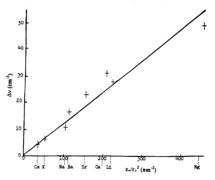
Figure 2. Plot of frequency pertubation  $\Delta v$  (cm<sup>-1</sup>) for a series of cations versus  $z_{+}/r_{+}^{2}$  (nm<sup>-2</sup>).
