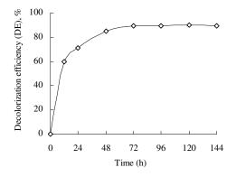
Figure 3. Effect of adsorption time on decolorization efficiency.
