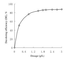
Figure 1. Effect of dosage on decolorization efficiency.
