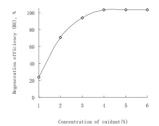
Figure 6. Influence of oxidant dosage on regeneration efficiency.
