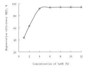
Figure 4. Influence of NaOH on regeneration efficiency.
