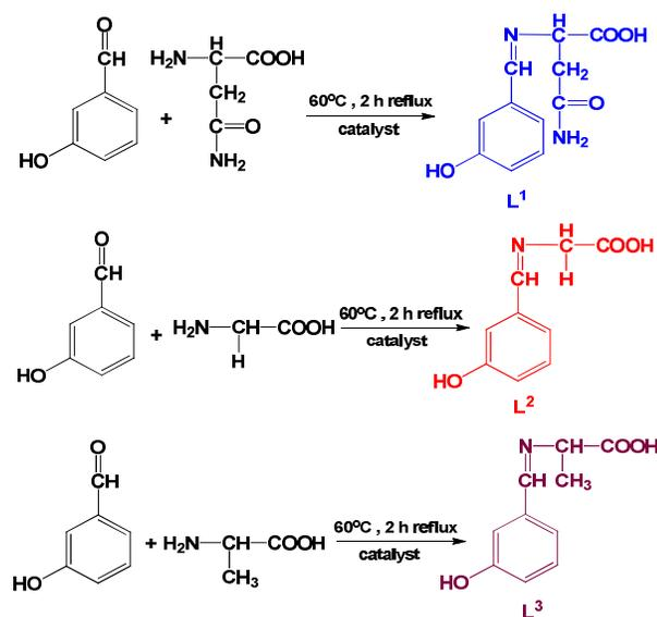
Scheme 1. Synthesis and the chemical structures of L<sup>1</sup>, L<sup>2</sup> and L<sup>3</sup>.
