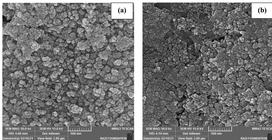
Figure 1. SEM image of (a)  $\text{Fe}_3\text{O}_4$  nanoparticles and (b) SDBS-coated  $\text{Fe}_3\text{O}_4$  nanoparticles.
