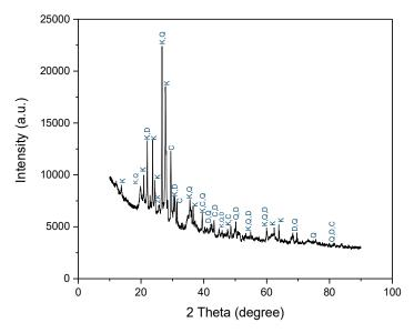
Figure 2. XRD pattern of sediment samples (K; Kaolinite (98-006-8697), Q; Quartz (98-003-1228), D; Dolomite (98-017-1524), C; Calcium Carbonate (98-042-3568)).
