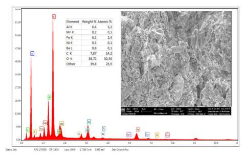
Figure 3. SEM images and EDX analysis of the sediment sample.
