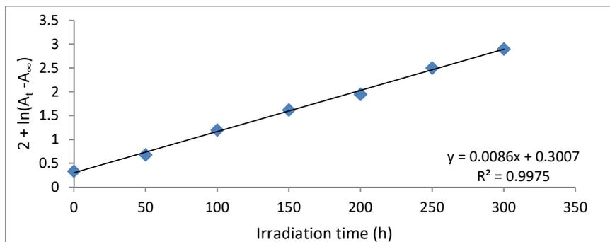
Figure 2. Changing in  $(A_t - A_\infty)$  versus UV irradiation time for blank PVC film.
