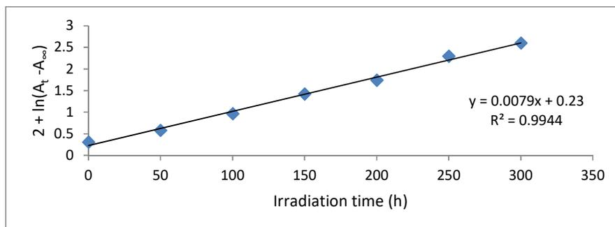
Figure 3. Changing in  $(A_t - A_\infty)$  versus UV irradiation time for PVC film filled with organotin(IV) number 5.
