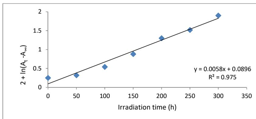
Figure 5. Changing in  $(A_t - A_\infty)$  versus UV irradiation time for PVC film filled with organotin(IV) number 3.
