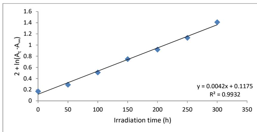
Figure 6. Changing in  $(A_t - A_{\infty})$  versus UV irradiation time for PVC film filled with organotin(IV) number **2**.
