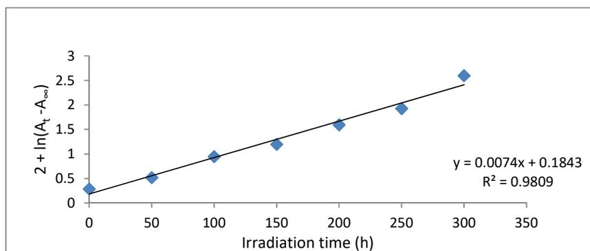
Figure 4. Changing in  $(A_t - A_\infty)$  versus UV irradiation time for PVC film filled with organotin(IV) number 4.
