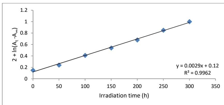
Figure 7. Changing in  $(A_t - A_{\infty})$  versus UV irradiation time for PVC film filled with organotin(IV) number **1**.
