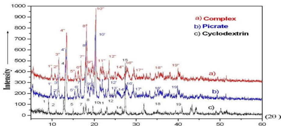
Figure 1. Experimental XRD patterns of **a)** the complex, **b)** the picrate and **c)** the  $\beta$ -CD.
