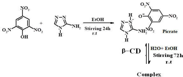
Scheme 1. Synthesis of picrate in first step and Synthesis of the inclusion complex of AT picrate with  $\beta$ -CD in second step.
