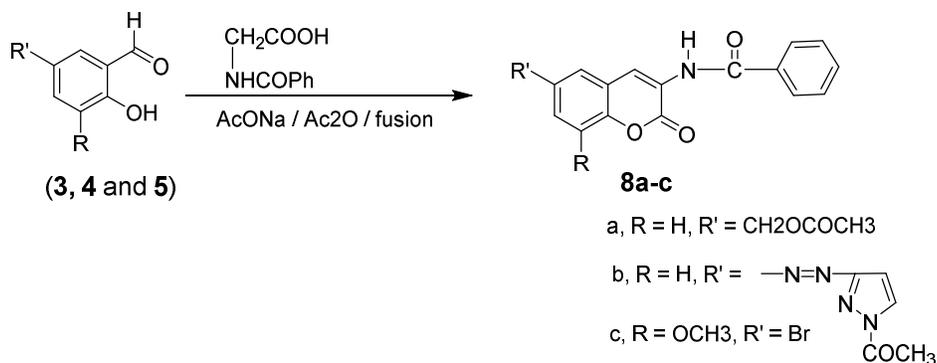
Scheme 2. Synthesis of N-(6,8-disubstituted coumarin-3-yl) benzamide derivatives (**8a-c**).
