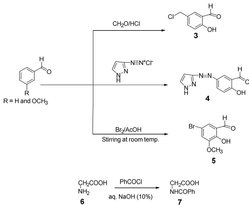
Scheme 1. Preparation of starting materials (**3**, **4**, **5**, and **7**) according to literature procedures.
