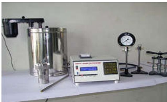
Figure 2. Bomb calorimeter used for the present work.
