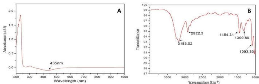
Figure 2. a) UV/Vis spectral characterization of green synthesized Ag-NPs. b) FT-IR characterization of green synthesized Ag-NPs.
