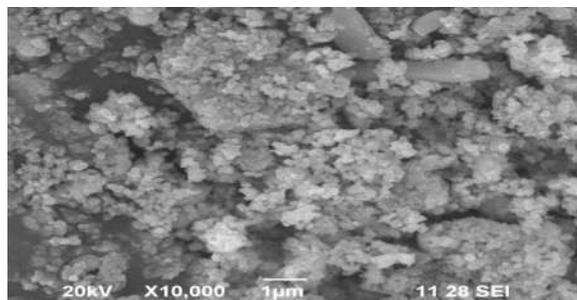
Figure 3. Scanning electron microscope images of synthesized Ag-NPs.
