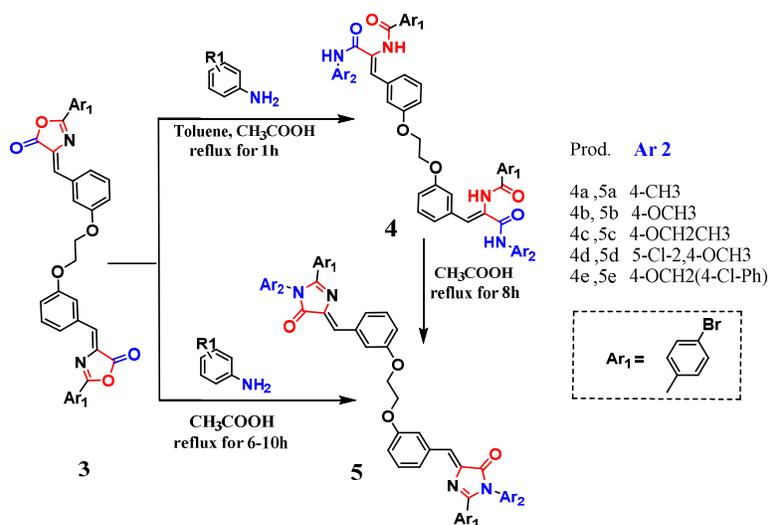
Scheme 2. Synthesis of bis-benzamide (**4**) and bis-imidazolones (**5**).
