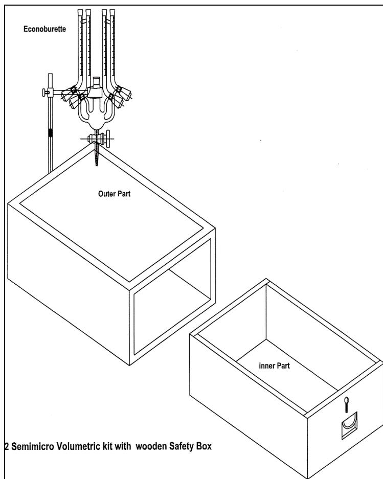
Figure 2. A sketch diagram of a wooden safety boxes for semimicro volumetric kit.
