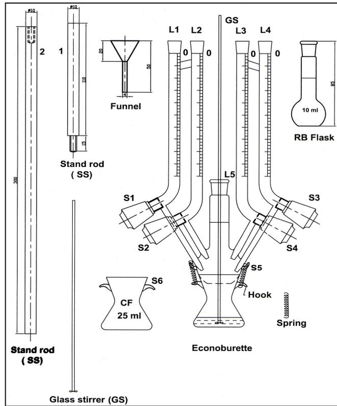
Figure 1<sup>\*</sup>. Sketch diagram of a semimicro volumetric kit: Spring model.
