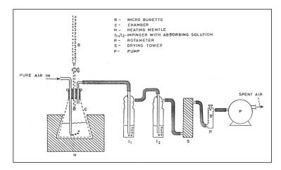
Figure 1. Assembly train for sampling of air pollutants.
