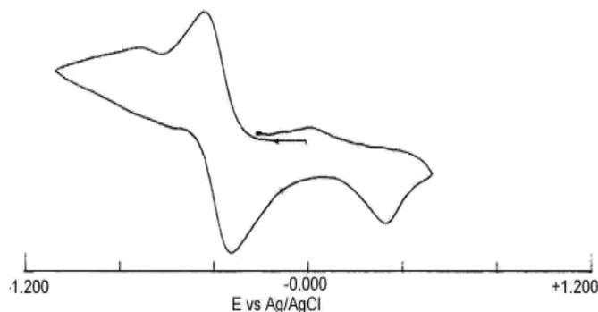
Figure 1. Cyclic voltammogram of type 3 complexes [(3), M = Mn, M' = H, B = C<sub>6</sub>H<sub>4</sub>] in DMSO at glassy carbon electrode (scan rate 200 mVs<sup>-1</sup>).
