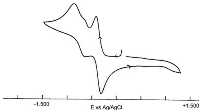
Figure 2. Cyclic voltammogram of type **3** complexes [(**3**), M = Mn, M' = Mo(NO)T<sub>p</sub>\*Cl, B = C<sub>6</sub>H<sub>4</sub>] in CH<sub>3</sub>CN at glassy carbon electrode (scan rate 200 mVs<sup>-1</sup>).
