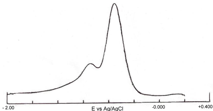
Figure 3. Differential pulse voltammogram of type **3** complexes [(**3**), M = Mn, M' = Mo(NO)T<sub>p</sub>\*Cl, B = C<sub>6</sub>H<sub>4</sub>] in CH<sub>3</sub>CN at glassy carbon electrode (scan rate 200 mVs<sup>-1</sup>).
