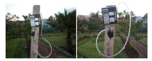
Figure 2. Sampling set up for TSP (left) and PM<sub>10</sub> (right).
