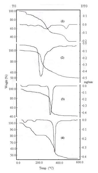
The obtained data for H[Sn(NTA)] (2) and H[Sm(NTA)]·H<sub>2</sub>O (3) complexes indicate that the decomposition reactions occurred as expected. The lattice water molecule in complex 3 is lost at a maximum temperature lying at 54 °C. The calculated weight loss of one water molecule in this complex corresponds to 5.04% in agreement with the obtained value of 5.50%. Since complex 2 contains no lattice water, it lakes such a step. The main degradation step for both
