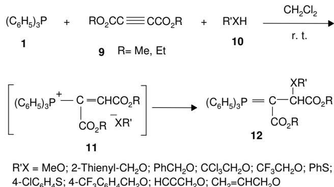
Scheme 2. Synthesis of highly stabilized phosphorus ylides **12** from dialkyl acetylenecarboxylates, R'XH **10** and triphenylphosphine [31, 40].
