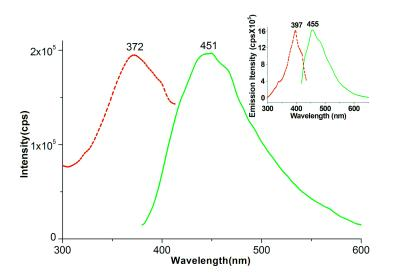
Figure 3. Solid-state photoluminescent spectra of 1 and pure isonicotinic acid (inset) at room temperature (Red: excitation spectra; green: emission spectra).
