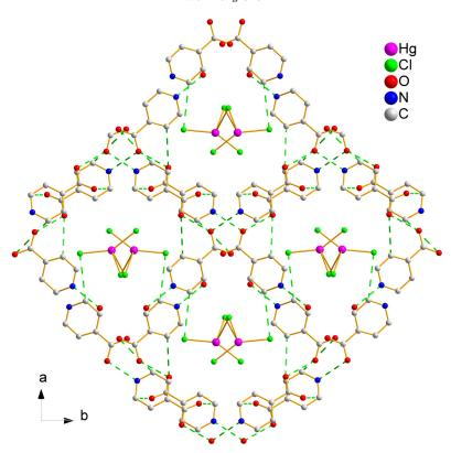
Figure 2. Crystal packing diagram of **1** with the dashed lines representing the hydrogen bonds. Distances of the hydrogen bonds in **1** (Å): O(1)-H(1A)···O(3) 2.555(3), N(1)-H(1B)···O(3) 2.712(4), N(2)-H(2A)···O(1W) 2.632(6), C(4)-H(4A)···O(4) 3.183(4), C(9)-H(9A)···O(4) 2.727(7), C(12)-H(12A)···O(1) 3.261(4), C(5)-H(5A)···O(2) 3.054(4), and C(10)-H(10A)···Cl(3) 3.560(8).
