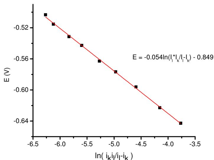
Figure 3. Plot of  $E$  versus  $\ln \frac{I_l * I_k}{I_l - I_k}$  for oxygen reduction at VPP-PEDOT modified GCE in oxygen saturated 0.5 M H<sub>2</sub>SO<sub>4</sub>.
