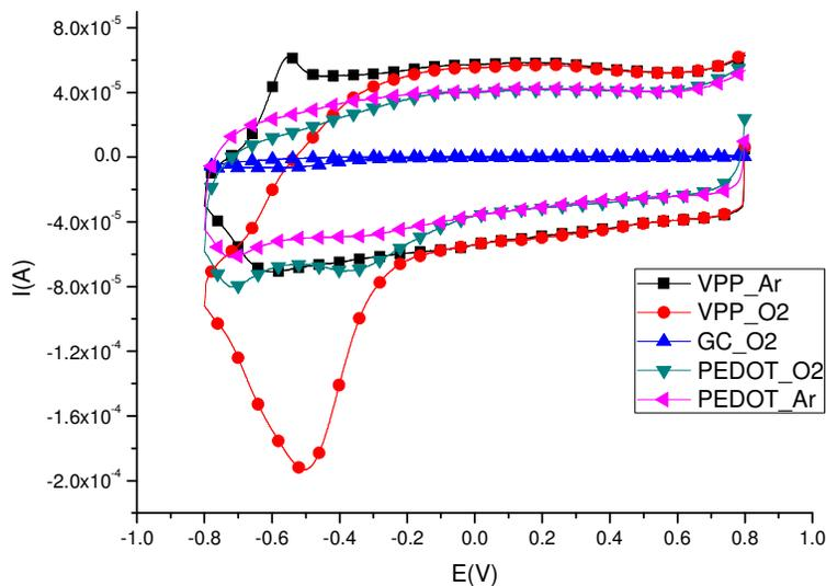
Figure 1. Comparative cyclic voltammograms of the modified and bare electrodes in oxygen saturated 0.5 M  $\text{H}_2\text{SO}_4$ . Scan rate 100 mV/s.
