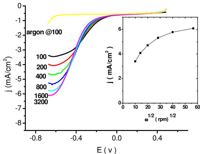
Figure 2. Rotating disk voltammograms at different rotation speeds for  $\text{O}_2$  reduction on a VPP PEDOT modified GCE in oxygen and Argon saturated 0.5 M  $\text{H}_2\text{SO}_4$ ; respectively, at scan rate of 10 mV/s between potential of 0.4 V to -0.672 V (*versus* Ag/AgCl). The inset shows Levich plot of limiting current at potential of -0.63 V (*versus* Ag/AgCl) for  $\text{O}_2$  saturated 0.5 M  $\text{H}_2\text{SO}_4$  at VPP PEDOT modified GCE.
