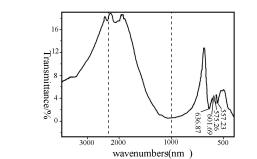
Figure 3. FTIR spectrum of LLZP.
