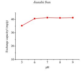
Figure 6. Effect of pH on the exchange capacity. Initial Na(I) ion concentration 0.01%(w/w), ion exchanger dose 1.00 g/100 g, time 200 min, agitation speed 200 rpm.
