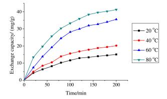
Figure 5. Influence of time on exchange capacity at pH 7.0, agitation speed 200 rpm.
