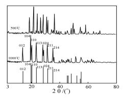
Figure 2. X-ray diffraction (XRD) scan of LLZP.
