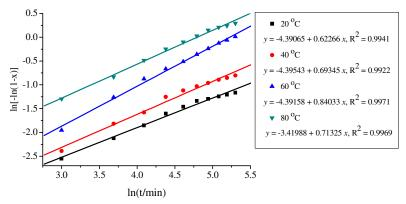
Figure 7. ln[-ln(1-x)] against ln(t) of Na/Li ion-exchange of LLZP.
