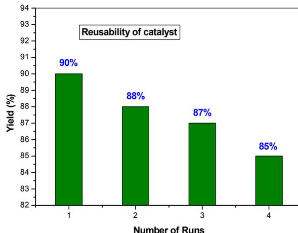
Figure 1. Recyclability of the catalyst: The SuSA catalyst could be reused four times without any loss of its activity towards the synthesis of 5,6-dihydro-2-(2-oxo-2*H*-chromen-3-yl)-5-phenyl-indolo[2',3':5,6]pyrano[2,3-*d*]pyrimidin-4(3*H*)-one.
