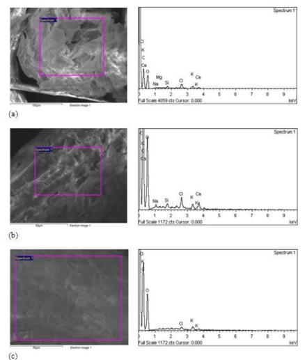
Figure 3. EDX images and elemental composition of (a) Ajwah, (b) Sukariah and (c) Jeddah.
