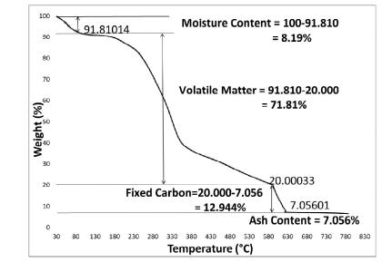
Figure 2. Percentage weight loss of DPF with temperature.
