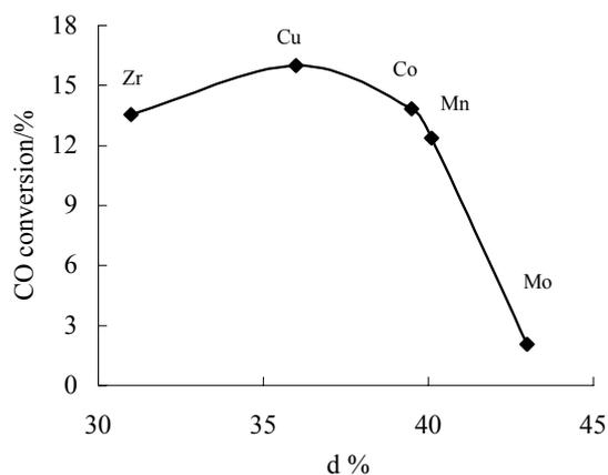
Figure 2. Correlation between d% of TM and catalytic activity.
