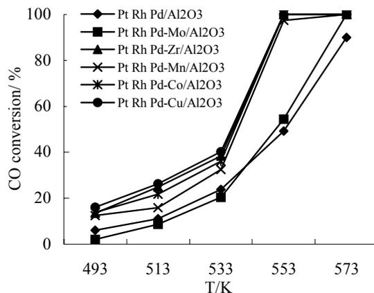
Figure 1. Effect of transition metal oxides on the catalytic activity for CO oxidation.
