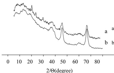
Figure 4. XRD patterns of the catalysts. a: Pt-Rh-Pd/ $\text{Al}_2\text{O}_3$  and b: Pt-Rh-Pd-1.56% Cu/ $\text{Al}_2\text{O}_3$ .
