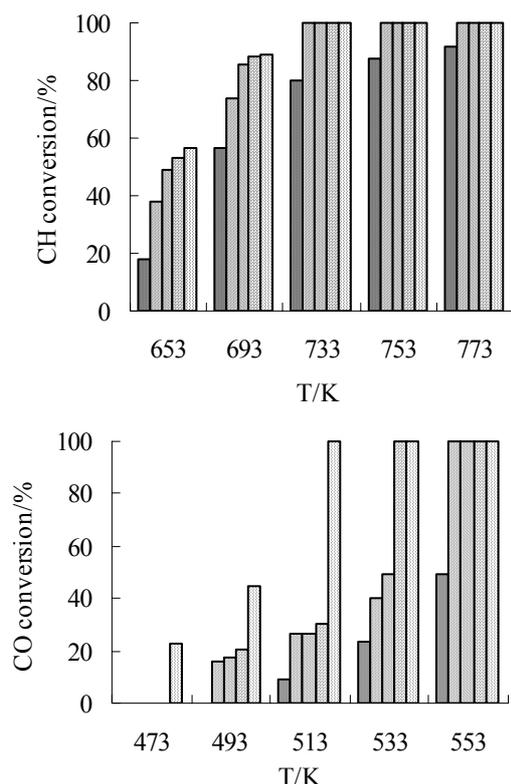
Figure 3. Effect of copper loading on the catalytic activity for CO and CH oxidation. ( Cu mol% ■ 0.00 ▨ 0.78 ▩ 1.56 ▪ 2.34 ▫ 3.12 % ).
