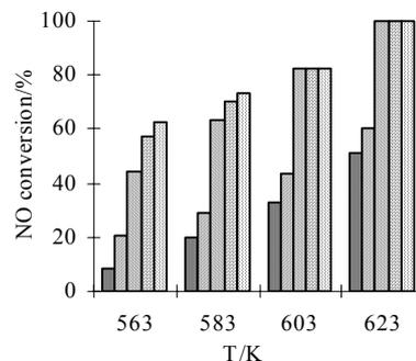
Figure 5. Effect of copper loading on the catalytic activity for NO conversion. (Cu mol%: 0.00%, 0.78%, 1.56%, 2.34%, 3.12%, respectively).
