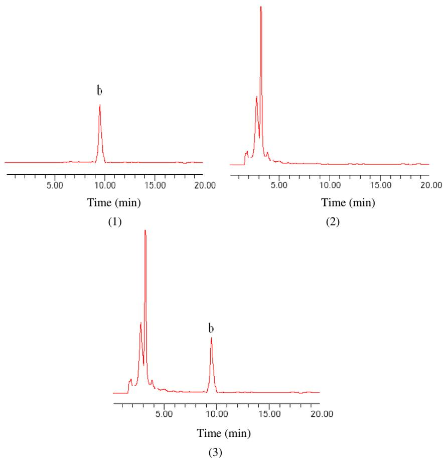
Figure 1. HPLC chromatogram of baicalin: (1) control of baicalin; (2) negative control of baicalin; (3) sample.
