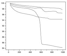
Figure 7. Thermogravimetric analysis (TGA) profiles of hydroxyapatites.
