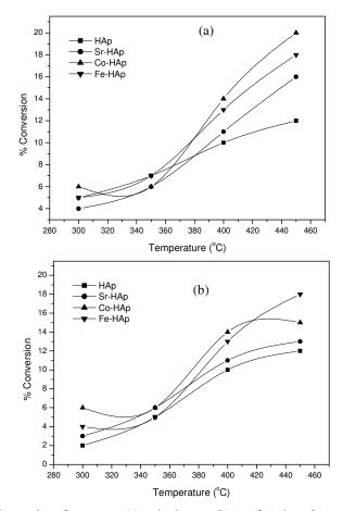
Figure 10. Conversion of *n*-pentane (a) and *n*-hexane (b) as a function of temperature.
