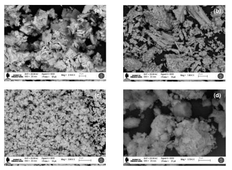
Figure 8. SEM images of (a) Co-HAp, (b) Sr-HAp, (c) Fe-HAp and (d) Hap.
