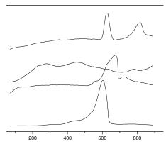
Figure 6. Temperature programmed ammonia desorption (TPD) profiles of hydroxyapatites.
