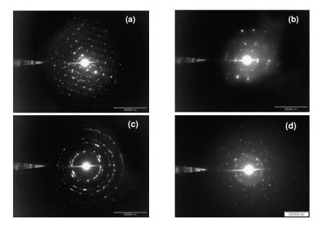
Figure 2. Selected area electron diffraction (SAED) images of (a) Co-HAp, (b) Sr-HAp, (c) Fe-HAp and (d) Hap.
