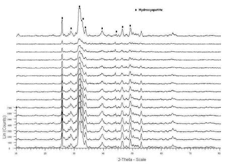
Figure 3. In-situ XRD diffractograms of HAp after reduction under hydrogen and re-oxidation.
