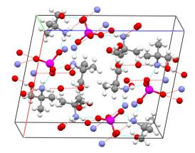
Figure 6. The crystal packing and the hydrogen bonding in the structure of  $OHRNH_{3/2}^{2+}(MOQ_{4})^{2-}$  (R = 2-methyl-1-propyl) crystalline molybdate salt.
