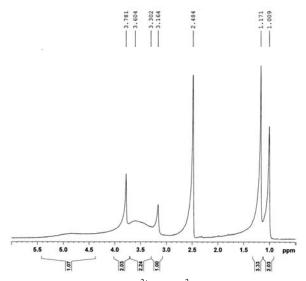
Figure 4. <sup>1</sup>H NMR spectra of  $(OHRNH_3)_2^{2+}(MoO_4)^{2-}$  (R = 2-methyl-1-propyl) as a new molybdate salt.
