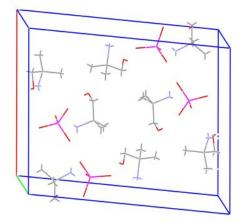
Figure 2. The crystal packing viewed along the b axis  $for(OHRNH_3)_2^{2+}(MoO_4)^{2-}$  (R = 2-methyl-1-propyl) as a new molybdate salt.
