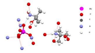
Figure 5. The hydrogen bonding in the structure of  $OHRNH_3)_2^{2+}(MoO_4)^{2-}$  (R = 2-methyl-1-propyl) as a new molybdate salt and the cohesion between the different groups is maintained by a three dimensional network of hydrogen bonds.
