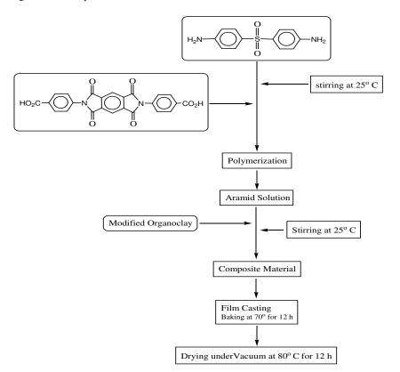
Scheme 3. Flow sheet diagram for the synthesis of PAI-nanocomposites film 5a and 5b.
