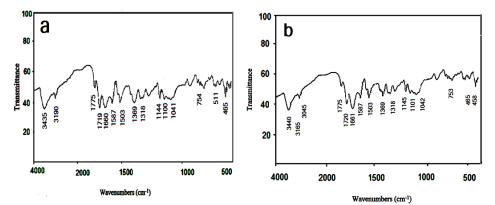
Figure 4. FTIR spectra of PAI-nanocomposite films **5a** (a) and **5b** (b).
