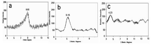
Figure 5. X-ray diffraction patterns of organoclay (a), PAI-nanocomposite films **5a** (b) and **5b** (c).
