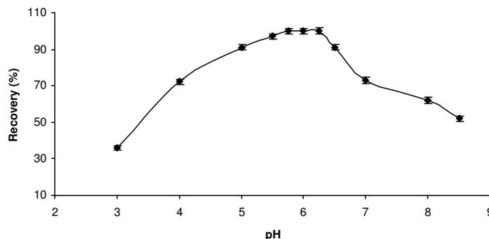
Figure 1. Effect of pH of the sample solution on the LL-DLLME extraction of lead. Conditions: Pb(II), 10.0  $\mu\text{g}$ ; ethanol, 2 mL; NaCl 10%(w/v), 1 mL and 1,2-DCB, 15.0  $\mu\text{L}$ .
