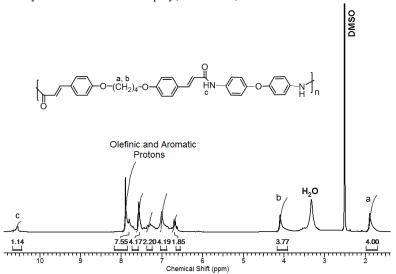
Figure 1. <sup>1</sup>H-NMR spectrum of OPEA **6e**.
