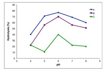
Figure 3: Effect of pH on hydrolysis of cassava starch by crude amylase of *Aspergillus sp* (A,C) and its mixed culture (B) at 65 °C
