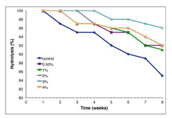
Figure 7: Effect of Cassava Starch as Stabilizer on Amylase Activity at 4  $^{\circ}\text{C}$
