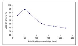
Figure 7: Lead removal with respect to lead initial concentration
