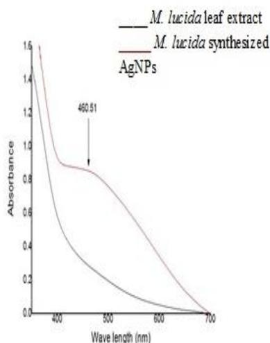
**Figure 3:** UV-vis Absorption Spectra of *M. lucida* AgNPs
