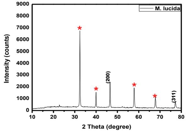
Figure 6: XRD diffractogram of *M. lucida* AgNPs
