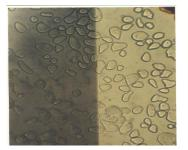
(a) Icacina trichantha starch oxidized (120 min)
