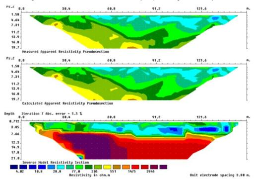
Figure 4: Inverse Model of Resistivity Section
