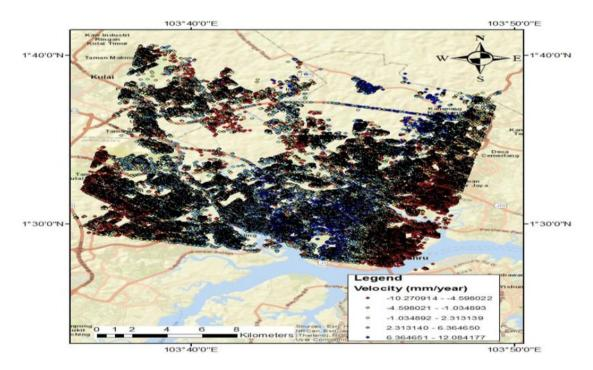
Figure 3: Persistent Scatterer Interferometry Map showing Ground Displacement.
