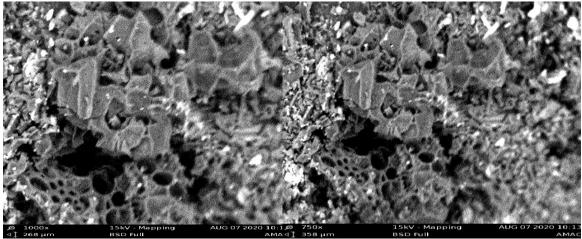
Figure 5: Scanning Electron Micrograph of AMAC/ H<sub>2</sub>SO<sub>4</sub> at different magnification
