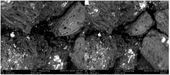
Figure 6: Scanning Electron Micrograph of BMAC/ NaHCO<sub>3</sub> at different magnification
