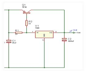
Figure: 6 Circuit Design of the Voltage Regulator
