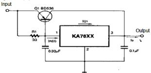
Figure: 4 The High Current Voltage Regulator [3]
