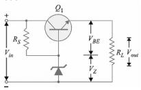
Figure: 2 Transistor Series Voltage Regulator [12]
