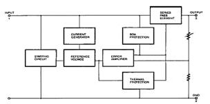
Figure: 3 LM7805 Internal Block Diagram. [3]
