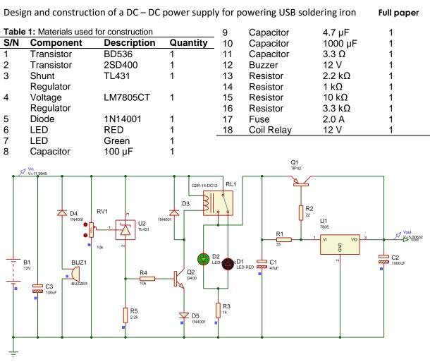
Figure: 7 Complete Circuit Design on Proteus
