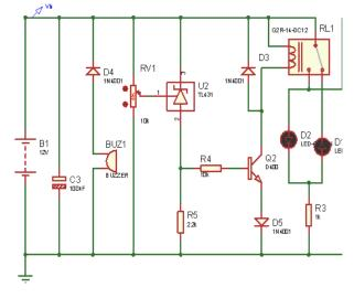
Figure: 6 Circuit Design of the Deep Discharge/Reverse Voltage Protection
