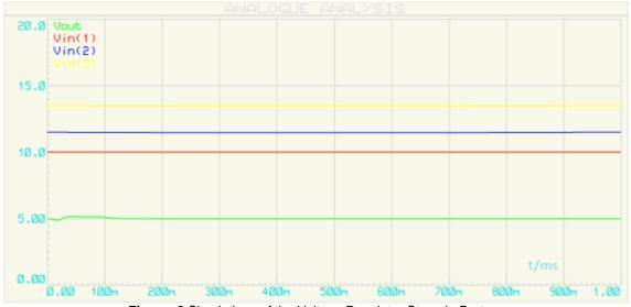
Figure: 8 Simulations of the Voltage Regulator Stage in Proteus
