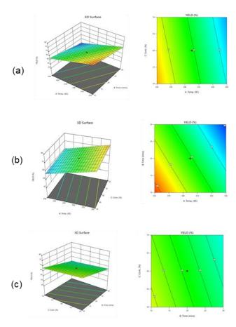
**Figure 9:** 3D surface and contour plots depicting the influence of process variables on the product yield of MGSAC (a. temperature and time, b. temperature and concentration, c. concentration and time).
