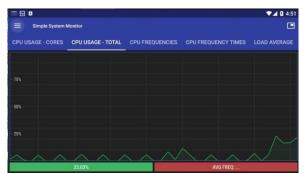
**Figure 8.** QPython 3L: Total CPU Usage of 23.03% on average while running python snippet.
