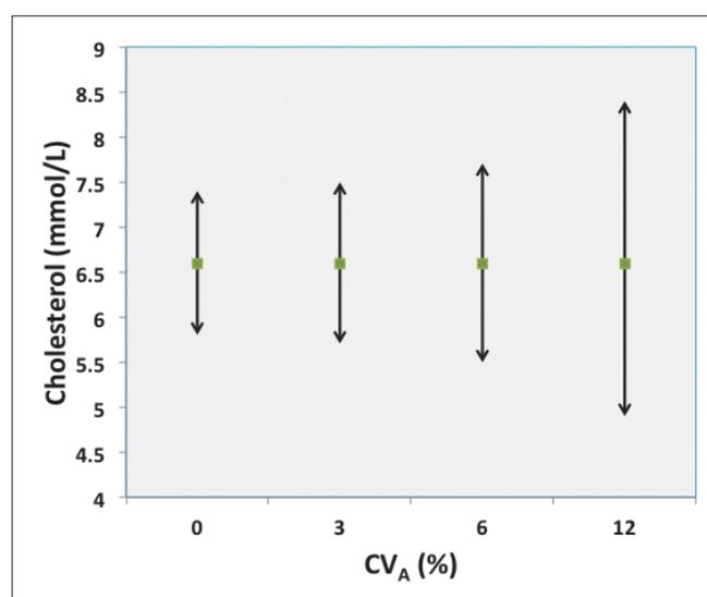
Fig. 2. With increasing analytical variation (represented by  $CV_A$ ), the uncertainty around the result obtained increases. The smaller the  $CV_A$ , the more precise the laboratory method and the more certain we are of the result obtained.
