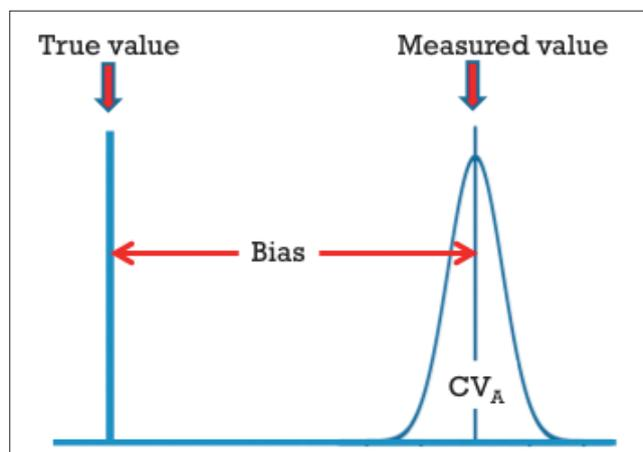
Fig. 1. Every result generated in the laboratory is associated with bias (systematic error) and imprecision (random analytical error –  $CV_A$ ).
