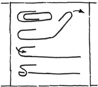
*Illustration 1. Lid retractor made from bent paper clip.*
