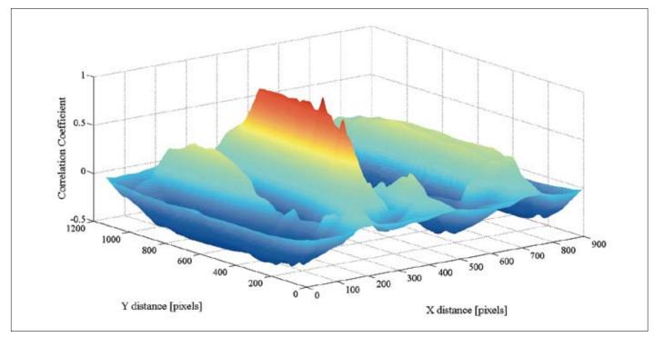
Fig. 2. A cross-correlation plot of two 2D images. The peak in red indicates the XY position at which the images have the best alignment.
