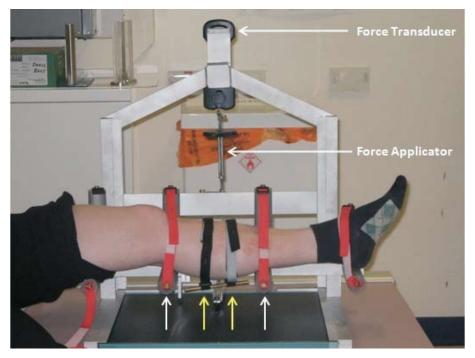
*Fig. 4. The four-point bending frame during an AP X-ray of a patient, showing the inner (yellow) and outer (white) fulcra, the force applicator and the force transducer.*
