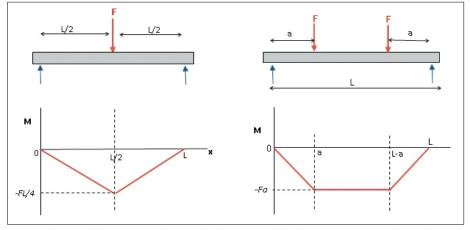
*Fig. 1. Schematic illustrations indicating the forces (F) and bending moments (M) for (a) three and (b) four-point bending configurations.*
